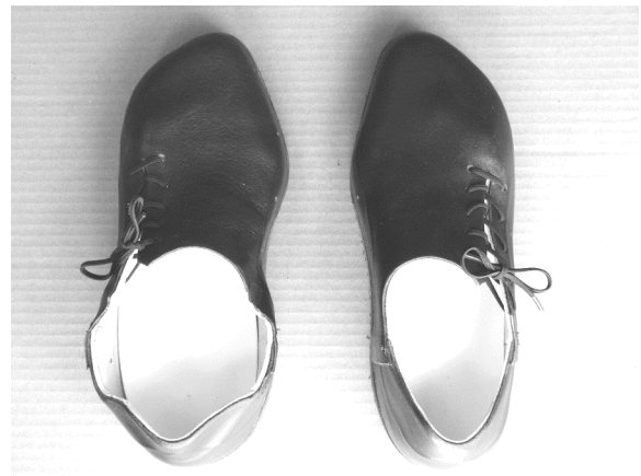
161 The finished shoes. The result was pretty good. But, I did have to make a small tuck in the side seams of the left shoe to tighten it just a little.
