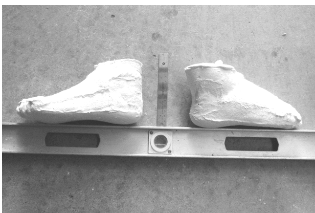
113 Look at my raw (un-cleaned) casts. Notice that the right knee could not flex properly while sitting. I will have to make some adjustment to the cast when turning it into a last. Take your time and look at these pictures with level and ruler.
