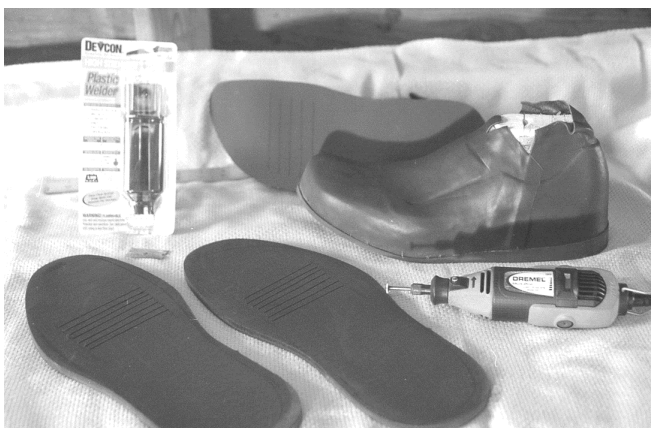
61 I bent the grooved soling, filled in the five minute epoxy and held the soling in position for five minutes. Then I put the original outer sole back on the shoes.
