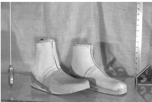
73 The right boot is for a customer with an amputation. The customer wants a walkable dummy front. This dummy is made from "mud".
