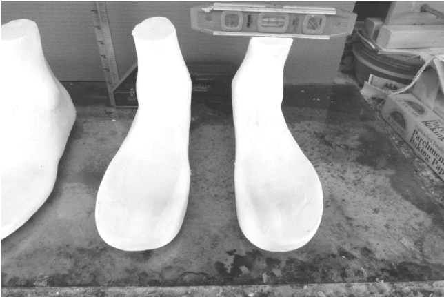
33 Use the level over and over again until the fabrication process is finished.
