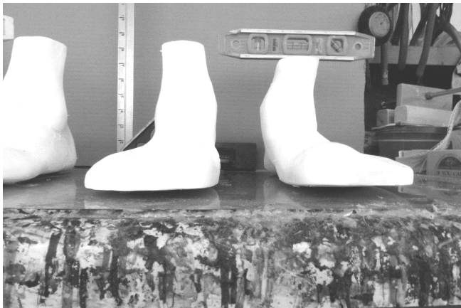
31 The level on top was derived from the vertical string and the judgment of artisan and/or craftsman.
