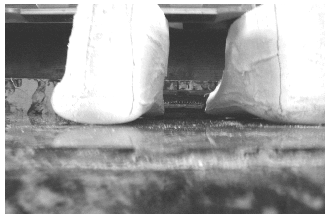
2 After the casting shell is poured up, the outer shell is removed. Be sure to mark the vertical string ridge with an indelible pencil. Try to mark it as straight as possible because sometimes it gets bent in the casting process.
