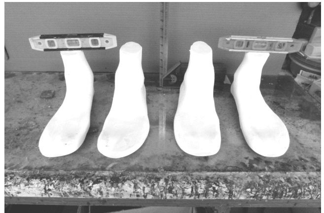
34 I use three levels. One for the bench top, one for the right last and one for the left last. They need to be in agreement.
