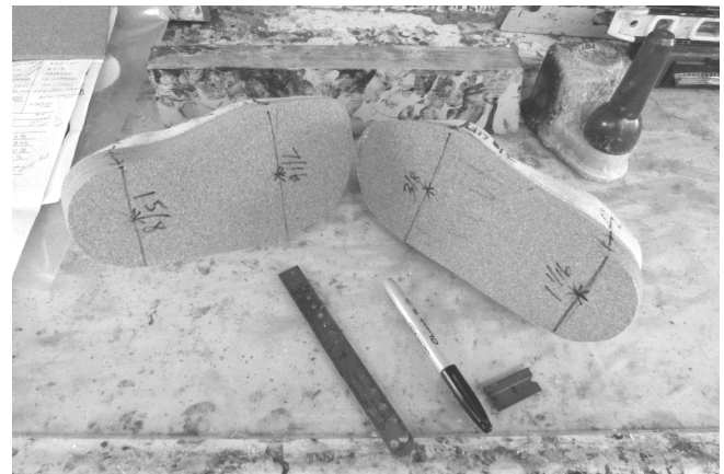
146 The cork has been sanded and measurements remarked.
