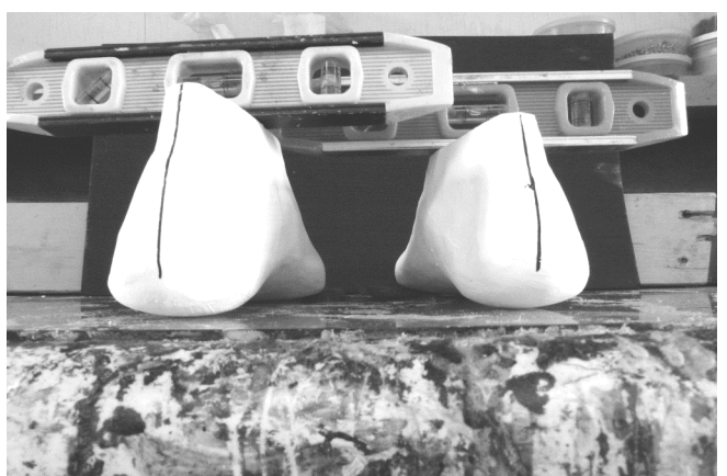
50 Ditto. The original vertical string has been replaced by the level on top of the cast or last. You get to use this reference all the time and it will help you make better shoes, boots and sandals.
