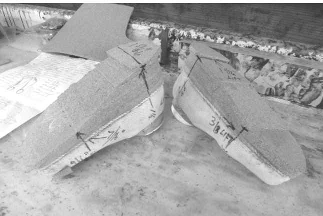
145 As I proceed in the construction process, I mark the necessary measurements and keep re-checking. These layers of cork are ready for sanding.
