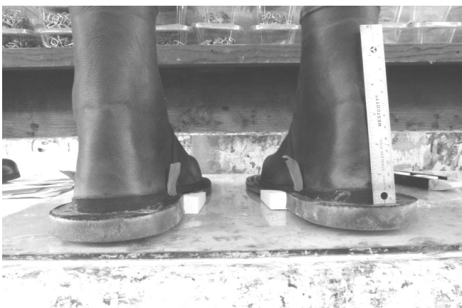
85 Actually, I put in a uniform thickness midsole and then added a small heel wedge filler.
