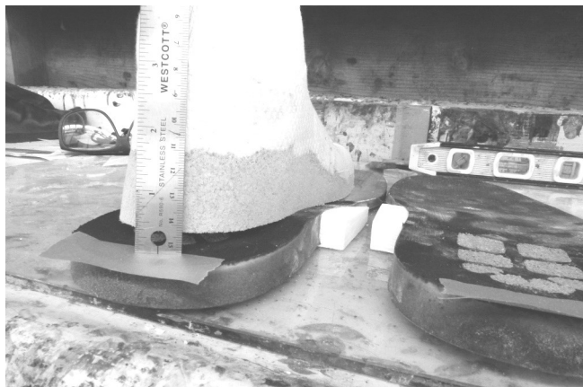
83 This picture is to give you a different angle of view from the previous picture. You can see that something needs to be sanded out or filled in to make the two surfaces match.
