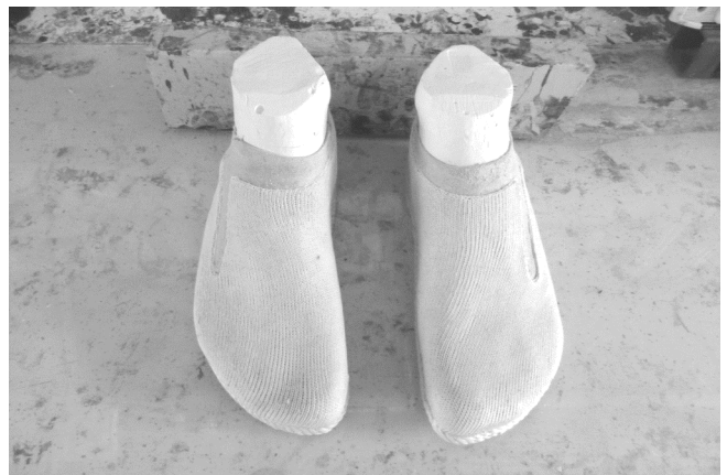
135 The measured blocks at the ball and heels are placed in the same location as the needle measurements. This is a top view so you can understand that when the base is finished, the blocks will be the base height measurements.
