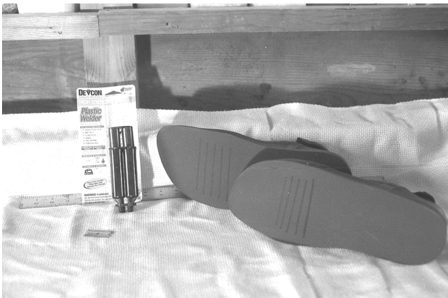
59 The podiatrist said he wanted more toe rock because he was acquiring a dropped foot condition (old age) and didn't want to trip. I cut these grooves so I could get the materials to flex and hold the new bend.
