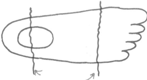
Arrows point to squiggly lines which represent saw cuts usually made with a hand dry wall saw.
