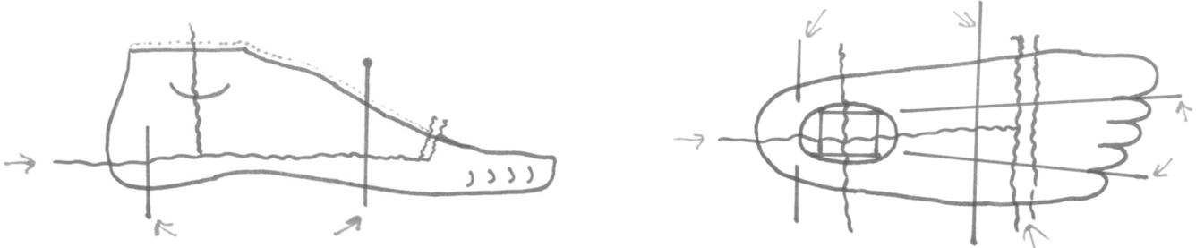
The arrows point to the pencil marks which must be aligned. Notice that the top pieces have been lowered the width of the saw cut. The front top piece has moved backward the width of as many vertical saw cuts as have been applied. Therefore, there is a gap at the front of the top piece which must be filled later. The front semi-vertical cut was made behind or to the rear of the mid point of the bunion joint. The back pieces at the heel should match flush.
