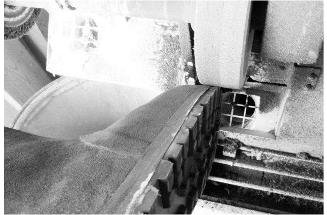
114 Sanding of outer edge of sole.
