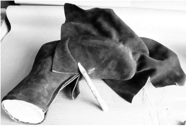
87 The leather is pressed in at side seam.
