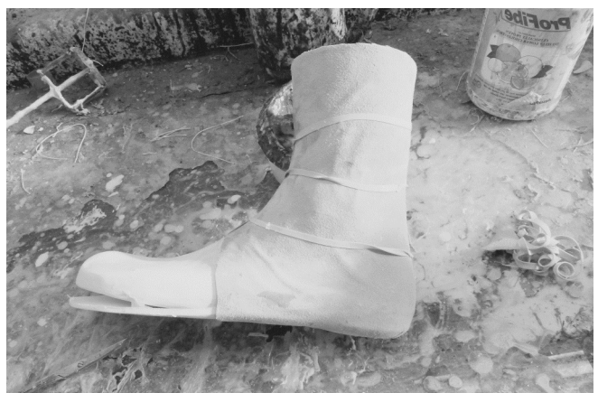
8 The lining leather is pulled and pressed to conform to the last. The latex is the binder or sticker. The wetting of the last keeps the latex from bonding so tenaciously to the last.
