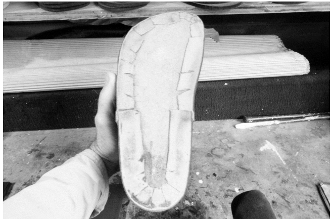
96 Inspecting the right boot underlap. Notice a little too much sanding at the heel.
