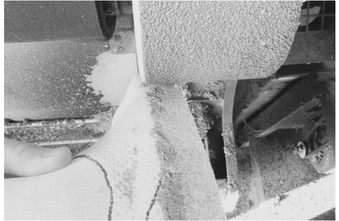
58 The dry edges of "mud" are sanded daily. Stop sanding as soon as the soft wet "mud" appears.
