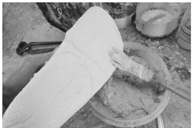
44 Latex is applied to the bottom.
