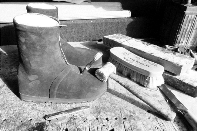
118 The bottom of center opening is punched.
