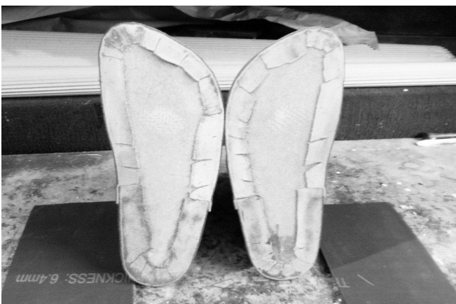
97 Inspecting the sanding of the underlap of both boots. Notice the width of boots across the ball and toe box areas. This customer needs custom made footwear for comfort and to prevent foot distortion by improperly sized footwear.
