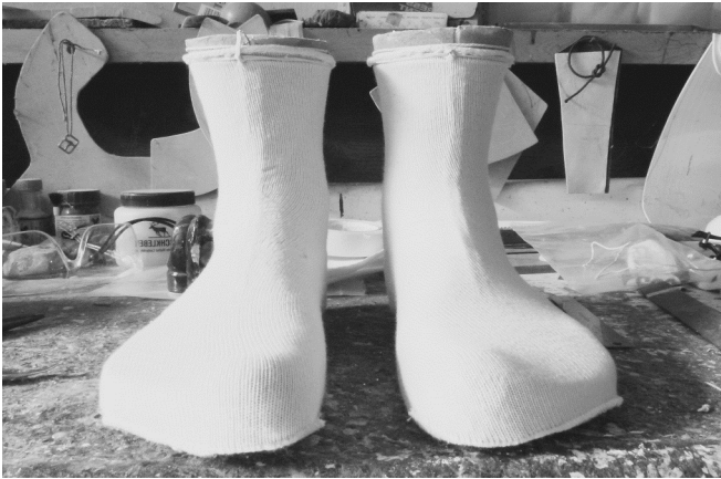
21 The lasts have been covered with a double knit (2 cotton threads) or a triple knit (2 cotton threads and 1 polyester thread) sock.
