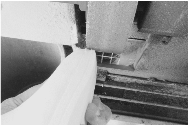
5 Both pieces of Pe-Lite® are trimmed, hand tacked to the last and sanded to fit the last.
