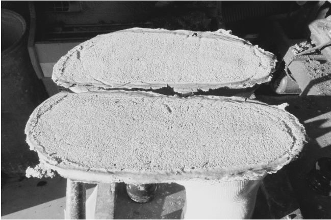
57 The boots with wet "mud" are allowed to dry 1 to 3 to 5 days with a fan and/or some sunshine.
