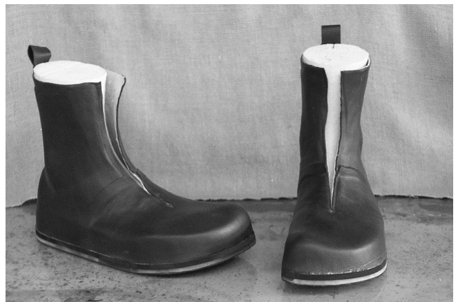
182 Mid and outer soles have been attached and pressed. The customer requested a flat soled boot without a heel wedge.
