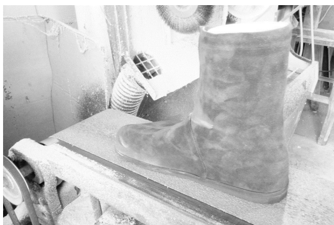
110 Finishing heel wedge on flat belt sander.
