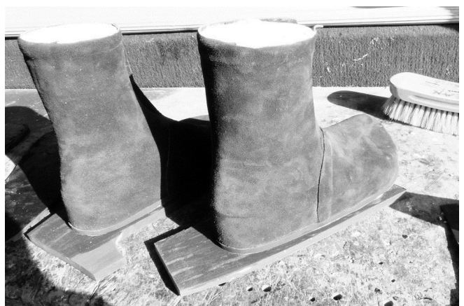
104 The craftsman didn't read the instruction on the work order! Not pictured is the removal of the outer sole by the use of thinner. A 5/8" or 30 iron heel wedge has been glued and pressed to mid sole.
