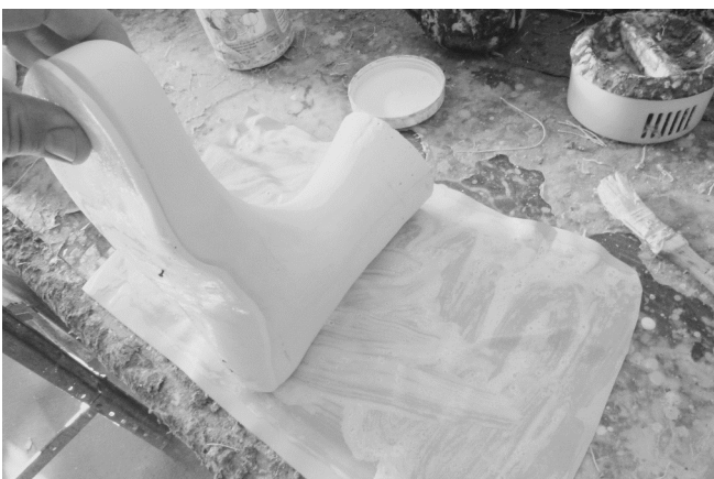
7 The boot last with inserts is usually soaked in water for 1 to 2 minutes and then placed onto the lining leather which has been brushed with latex.
