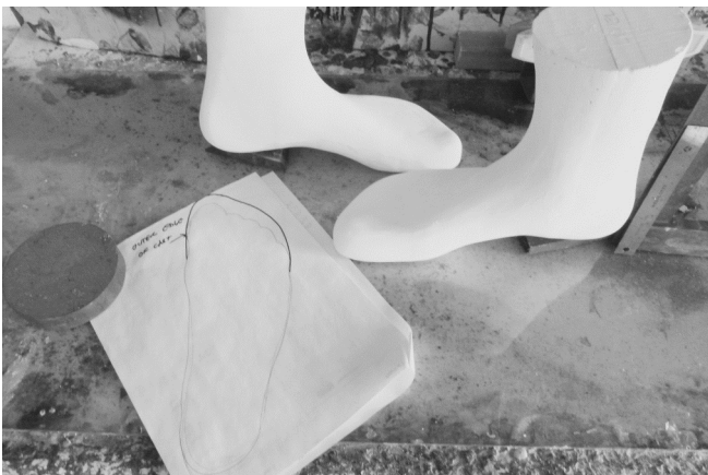
1 The completed boot last is compared with the elongation drawing taken at the time of casting.
