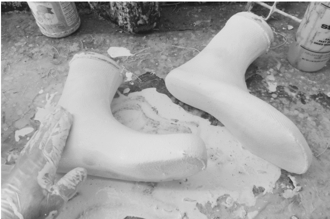
23 Ditto and press out the excess latex.
