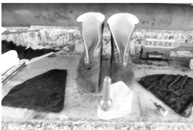
133 Gluing the tongues to boots.
