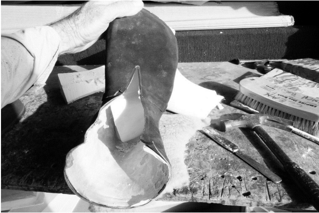
123 Trying to get the front of last out of boot.
