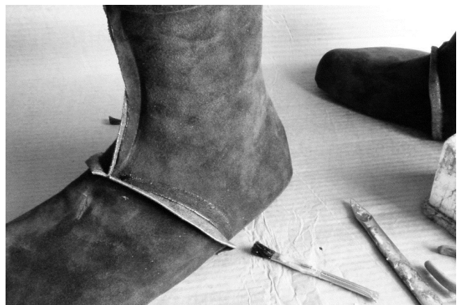
92 Adhesive is applied to the side seam areas.
