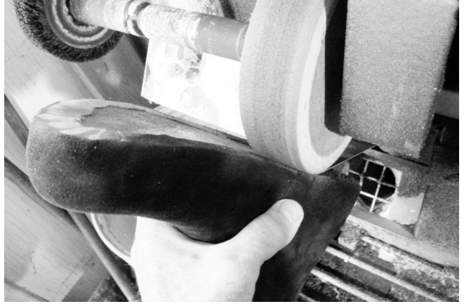
94 The underlap is sanded carefully!
