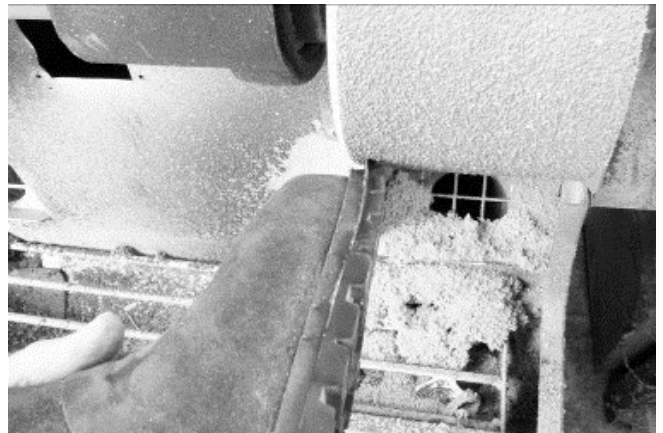
102 The outer edge of outer sole is rough sanded.
