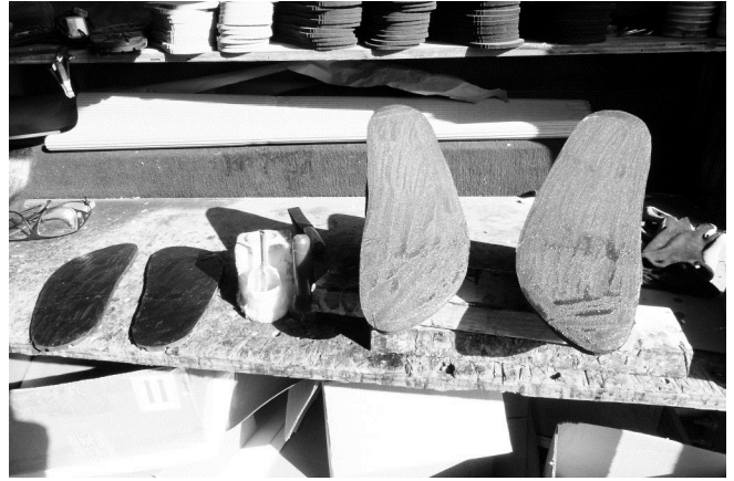
112 Gluing of outer sole.
