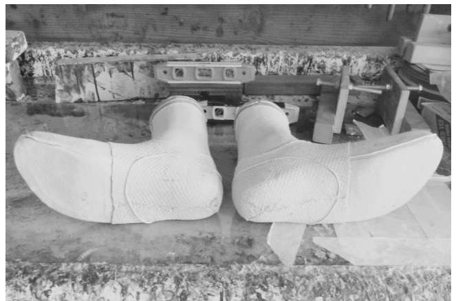
32 A design cord is applied to mark a heel counter and an arch to toe box stiffener of Monks Cloth.
