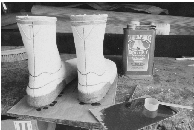
73 Applying fiberglass resin to heel counter base in order to strengthen the outside walls of the dried "mud".
