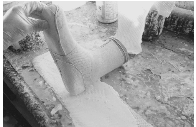
36 The Monks Cloth heel counter is latexed and applied.
