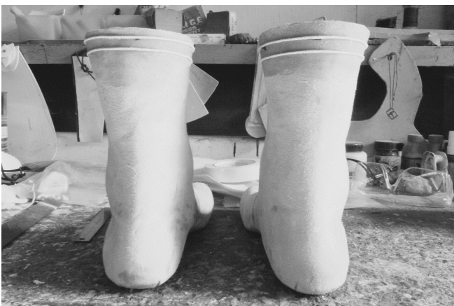
19 The "good" artisan takes time to recheck and adjust the stance of last and position of design cords.
