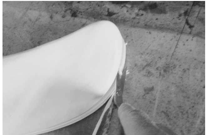
6 The feather edge of top layer of firm density Pe-Lite® is trimmed off.
