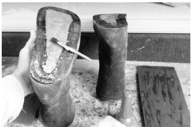
98 Applying two coats of glue to the bottom underlap and one coat to the mid sole.
