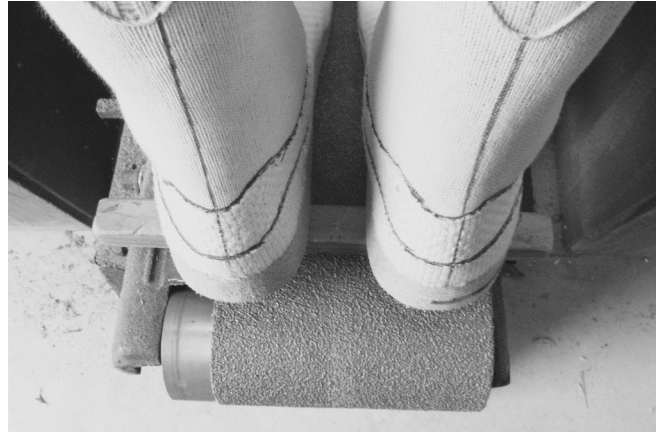
70 Comparing right and left boot. Checking roundness and uniformity of "mud" around outside edge of heels.
