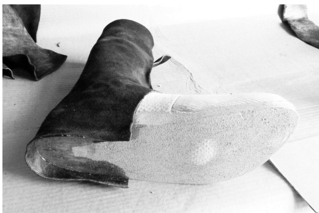
83 The bottom leather underlap is cut to size.
