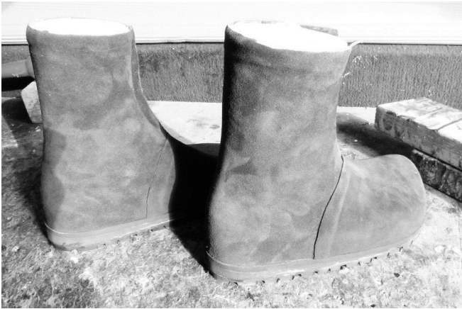
113 Outer soles have been attached and pressed.
