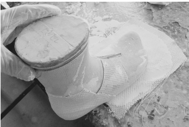
37 The Monks Cloth bottom front arch to toe box stiffener is latexed and applied.
