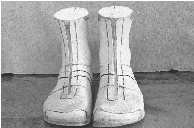
171 Location of toe box bumper protection area such as extra layer of Monks Cloth, shoe goo®, polyurethane treatment, or fiberglass resin.
