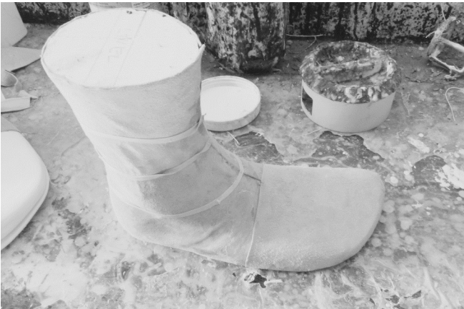
12 The front lining leather is applied to the last.
