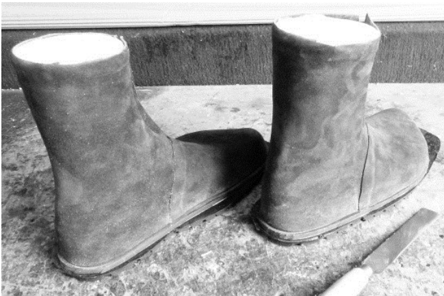
101 The outer sole is attached and pressed onto the mid sole.
