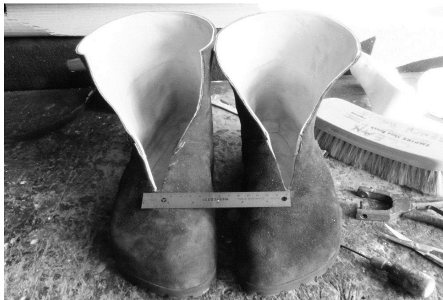
130 Measuring the uniformity of lace openings and eyelet holes.
