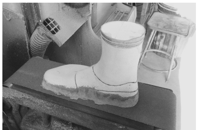
62 Sanding bottom of "mud" carefully!
