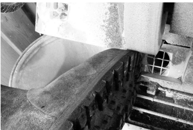
103 The edge of sole is smooth sanded.
