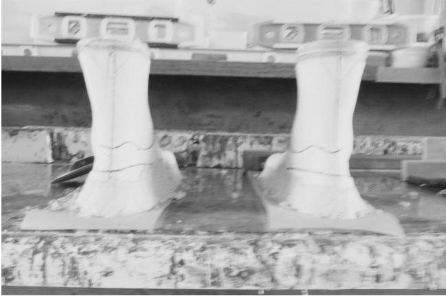
51 If needed, the boot is weighted to maintain the level. Notice weight placed on left side of left boot.
