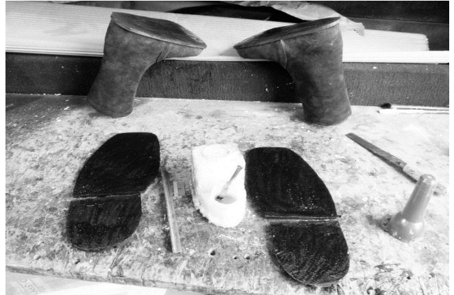
100 Adhesive is applied to mid sole and outer sole.
