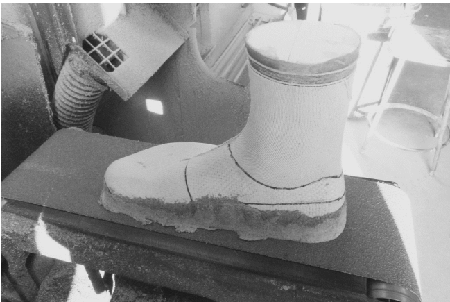
59 The dry bottom is sanded daily. Stop sanding as soon as the soft wet "mud" appears.
