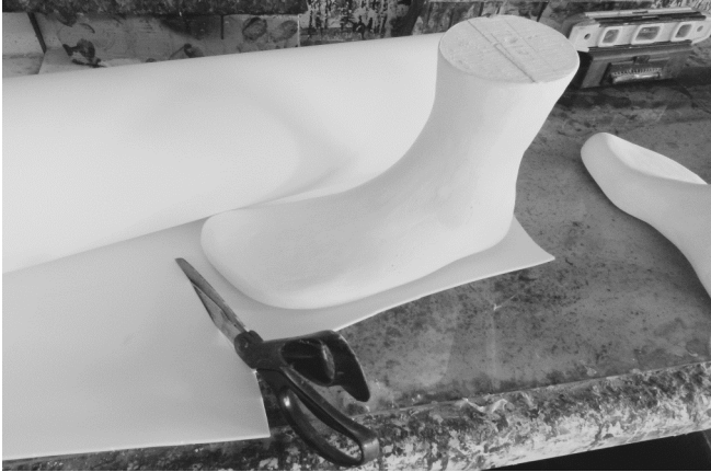
3 A layer of 3mm Pe-Lite® firm density is cut to size and an additional layer of 3mm Pe-Lite® medium density (not pictured) is cut to size.
