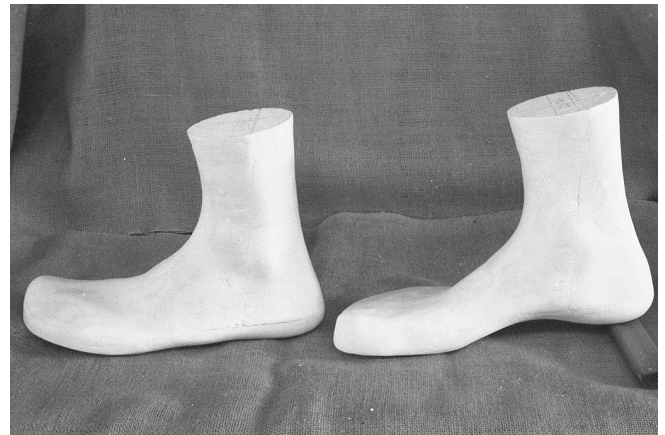
144 This picture is to help you to consider the heel and toe box lifts before the shoe or boot is made. If the angles are good, they will have a positive contribution to the comfort of the wearer.
