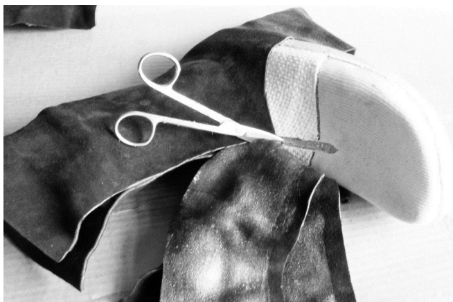
81 Ditto. Notice the leather is applied inside out or rough side out as requested by customer.
