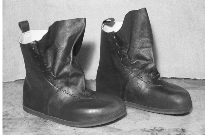
184 The tongues have been bonded, stitched and rivet holes have been opened.
