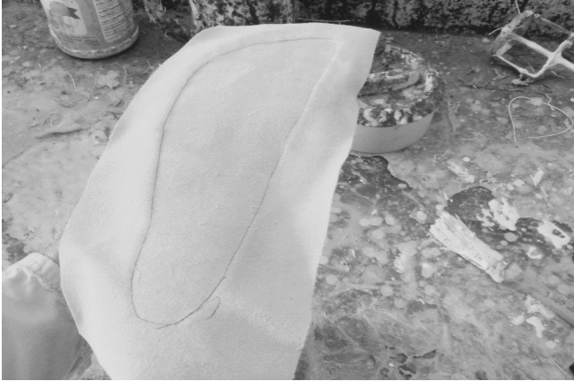
15 Bottom lining leather is applied.
