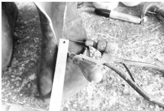
132 Measuring distance between eyelet holes.
