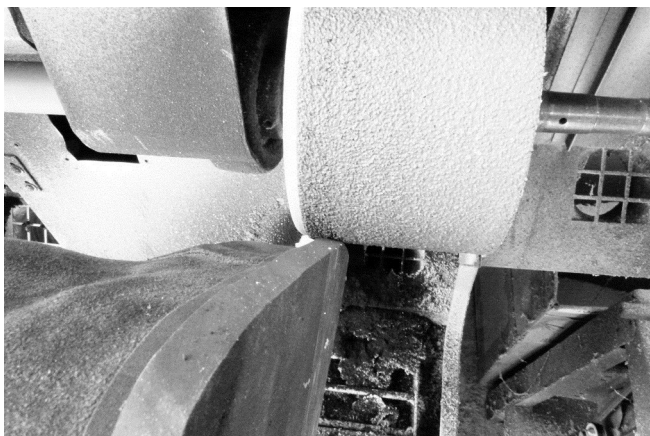
105 Sanding of heel wedge for 5/8" lift at heel and 0" at ball of foot.
