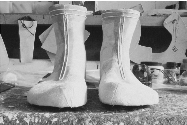
17 Design cords are applied to lining leather to mark top of boot and front opening.
