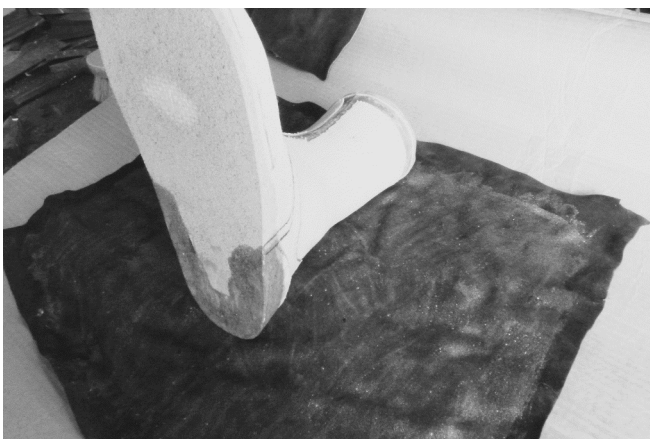
79 Leathering back of boot using adhesive as a bonding agent. Glues or latex are both acceptable but have different properties and attributes. This pair of boots was done with Ortex®.
