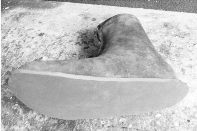
99 The mid sole is attached and pressed.
