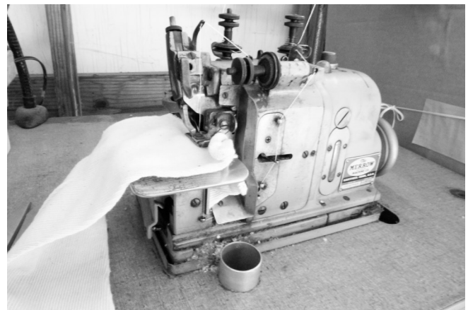
The Marrow sock seaming machine. This machine is used to sew the toe closing seam.
