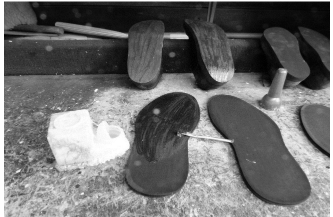
8 Applying adhesive to bottom of shoe and outer sole. Contact cements have an open time (wet time) and need to become tack free (not sticky to the touch). Some adhesives perform better if re-heated.
