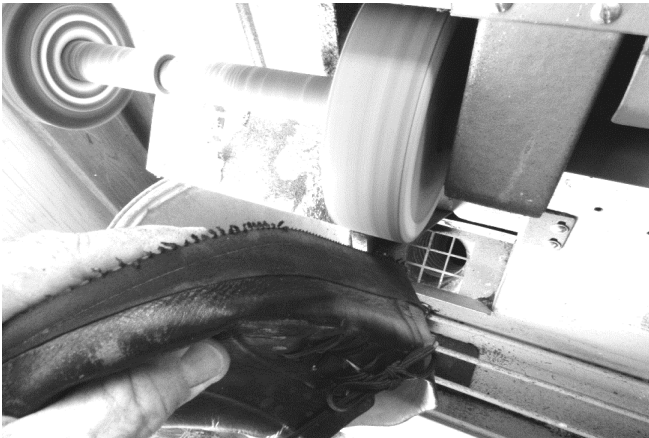
13 Remove the edge feathers by lightly, very lightly sanding at a slight angle and usually go in the opposite direction.
