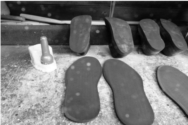
7 Sand top of outer soling if necessary to clean dirt, dust and grime which will interfere with good bonding. Blowing off with compressed air just before applying adhesives is a good habit.
