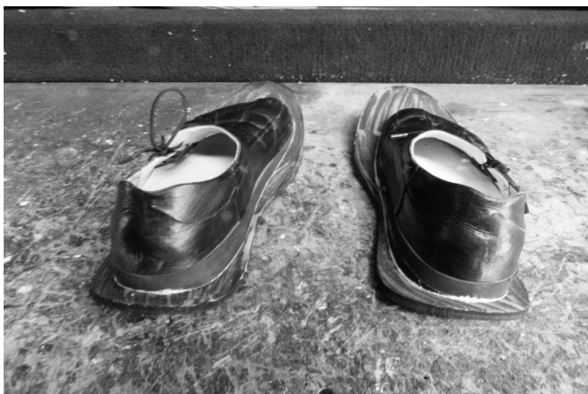
9 When the adhesive is ready, carefully position the shoe over the outer sole and then place it onto the outer sole. If you make a mistake in placement, you need to remove the sole. Go back to picture #1 and use thinner to de-bond it.
