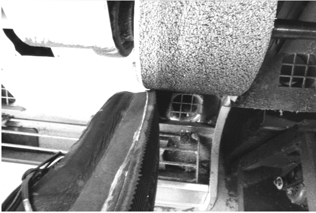
11 The outer edge of soiling is carefully rough sanded. Many workers at shoe repair shops are not good sanders. Quality sanding takes good hand and eye coordination. It is not the time for multi tasking or listening to the voice box.
