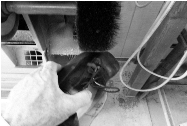
19 Brush the sole too. Finishing with a hand brush, and sometimes a soft cloth, with or without a slight amount of moisture, will help to produce a superior shine.
