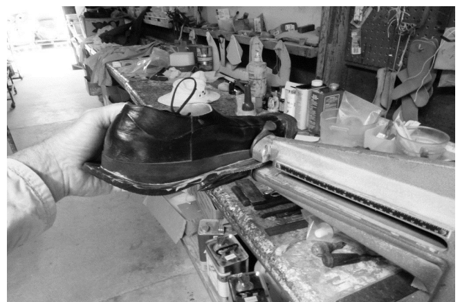
10 The excess outer soling is trimmed with a simple trimming machine or a sharp trimming knife.
